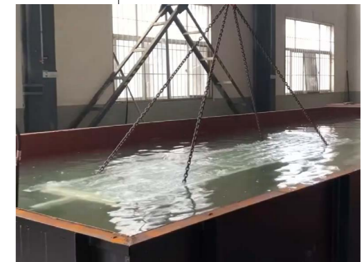
Coil leakage test
